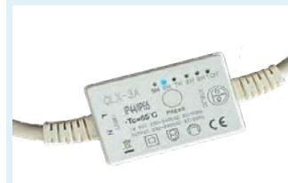
At the touch of a button, select 5, 6, 7, 8, 9 or 10 hrs of operation then an automatic switch-off. Octoplus compatible.
